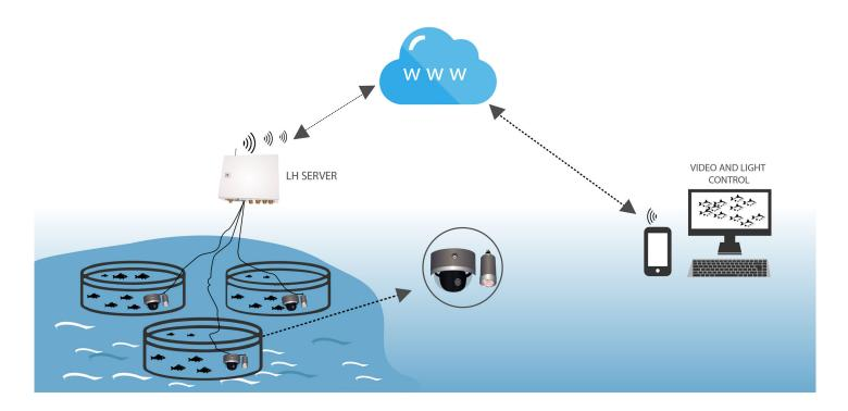
LH video server for Live view of up to 8 x underwater camera on PC or smartphone.
